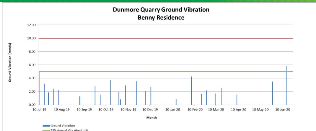
Figure 13 FY20 Ground Vibration Monitoring Data
