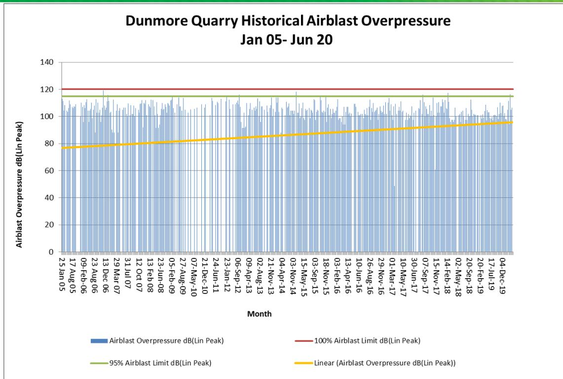
Figure 15 Historical Airblast Overpressure Monitoring Data
