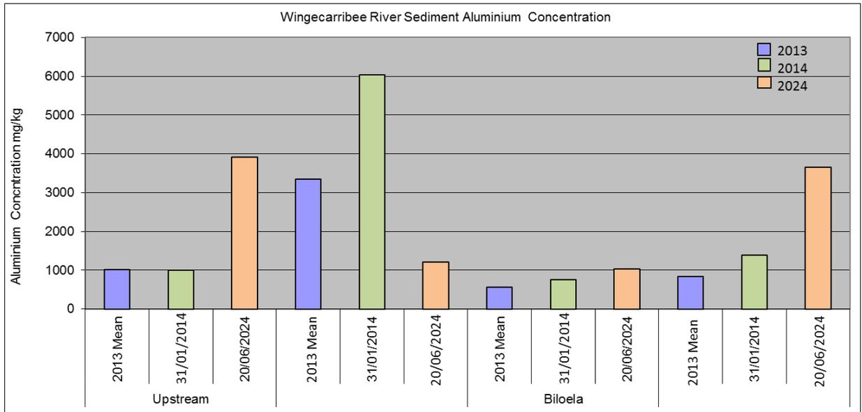
**Graph 7 - Concentrations of Aluminium (mg/kg) in River Sediments**
