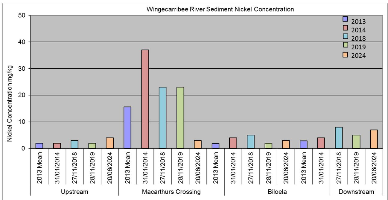
**Graph 10 - Concentrations of Nickel (mg/kg) in River Sediments**
