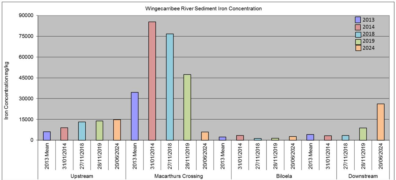
**Graph 8 - Concentrations of Iron (mg/kg) in River Sediments**
