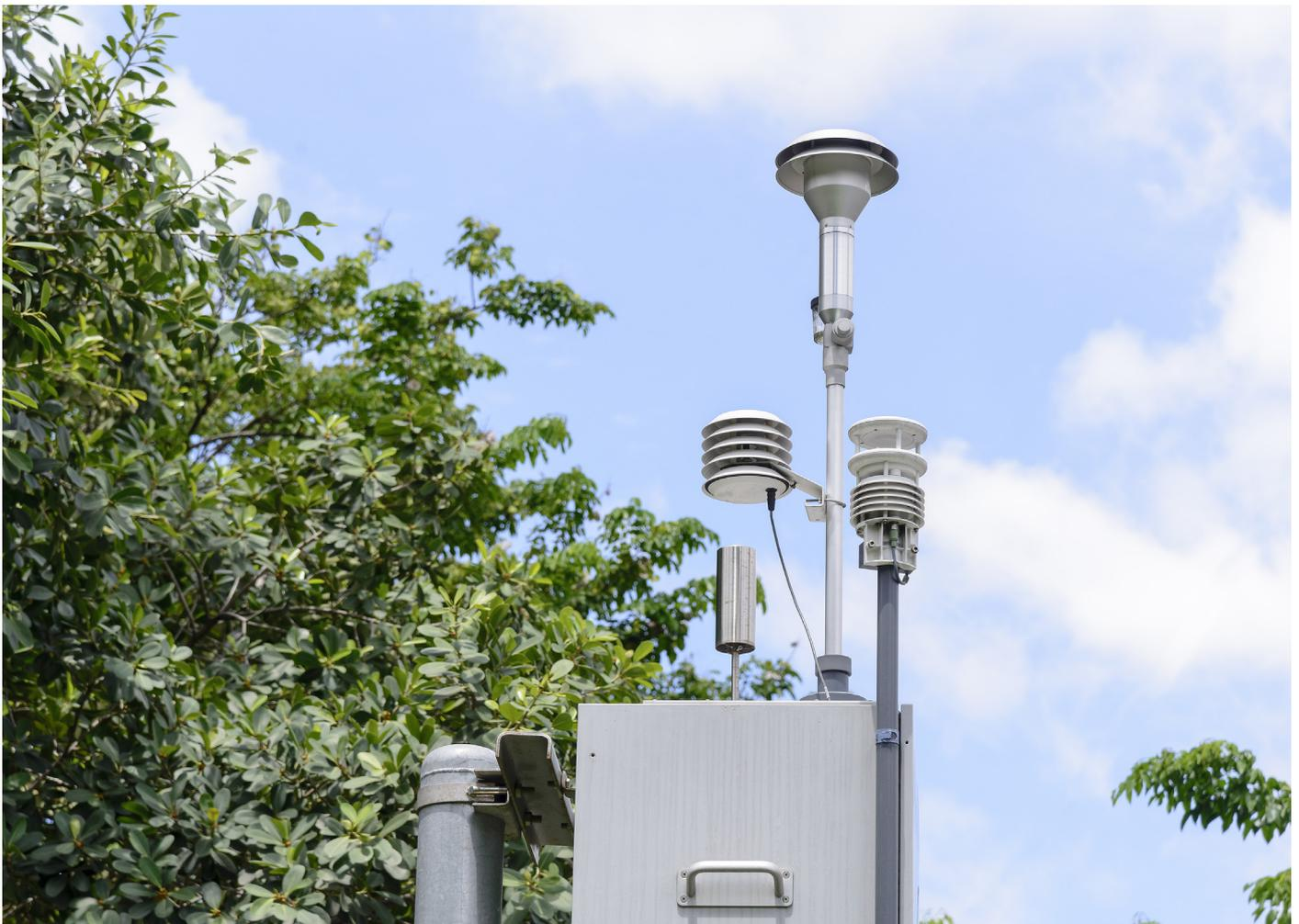
Example of air pollution detectors used for measuring air quality
