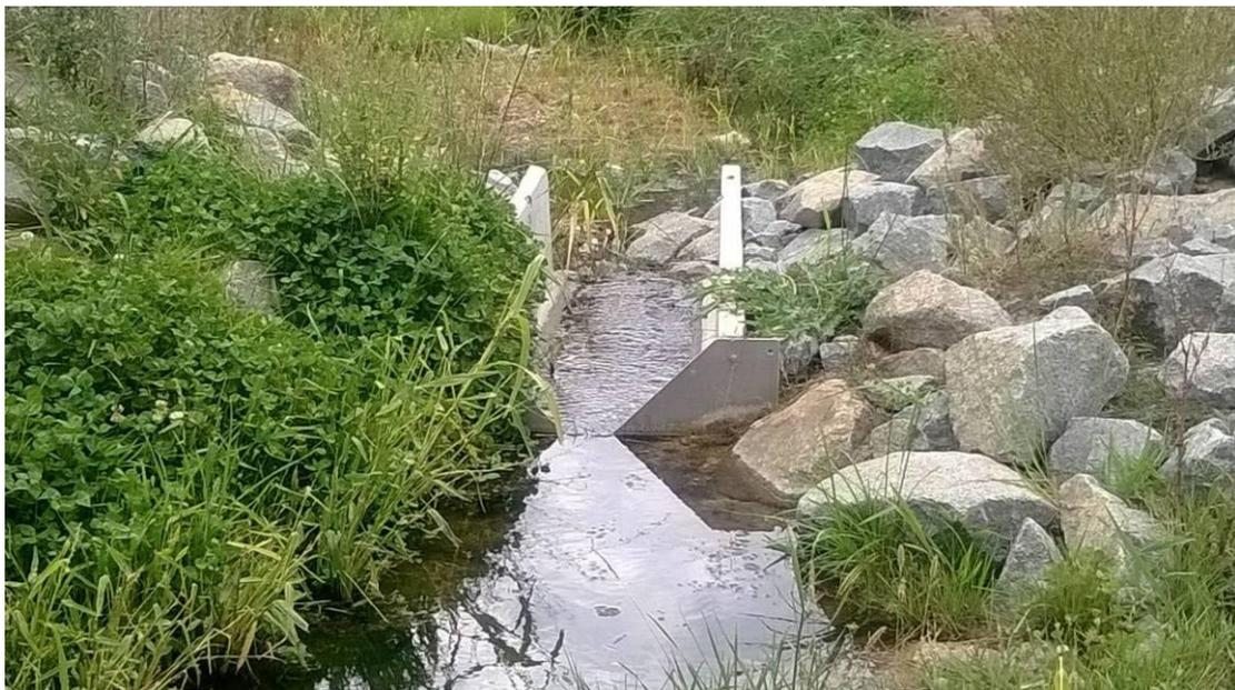
**Plate 7 - Water flow Measurement in Tangarang Creek**
