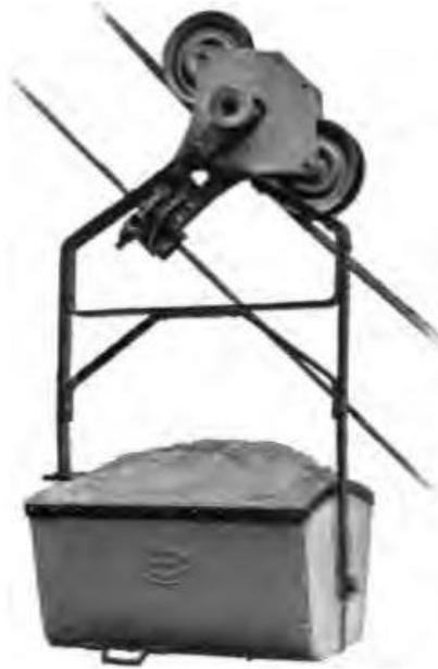
Fig. 12. Carrier, with Bleichert Patent Automatic Underhung Grip.
