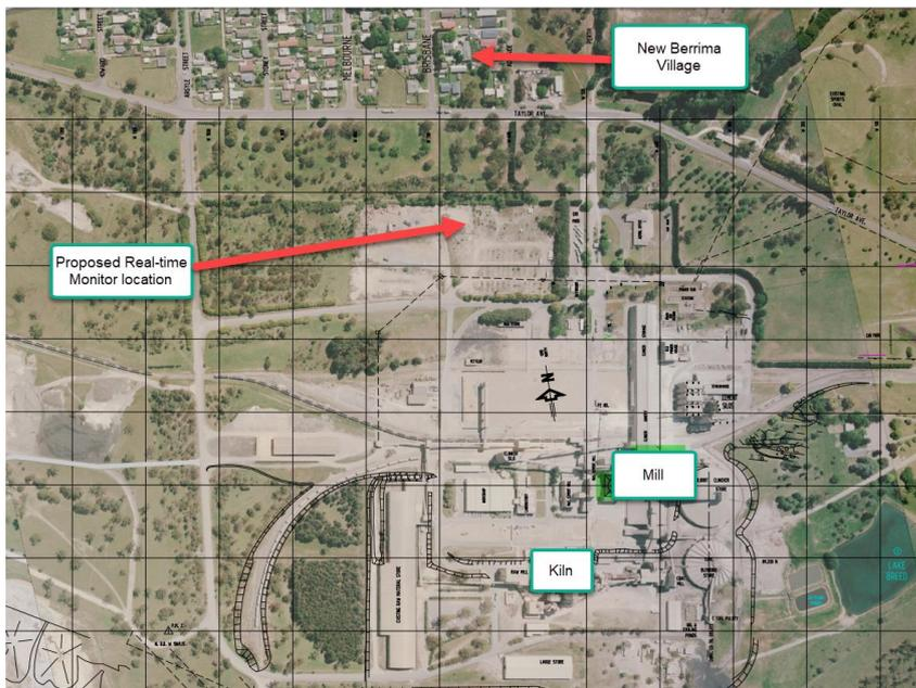
Figure 3 – Trial real-time dust monitor location
